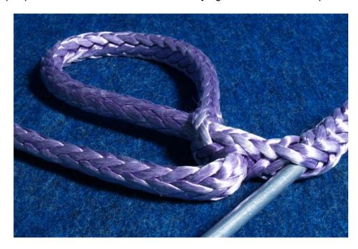
Push the metal fid down the center of the rope being careful not to snag any strands. Run the fid down the rope slightly farther than the buried length determined earlier. Pull the metal fid out of the rope.
