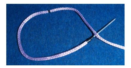
Care must be taken to ensure that the insertion has 6 strands on either side of fid
