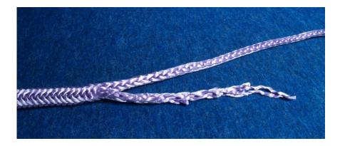
At this point, readjust eye to correct size, and check that lockstitches are even.
