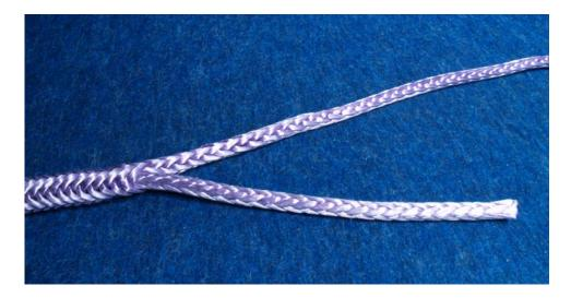
Strands are to be tapered in a matched "S" and "Z" pair. The first pair to be matched are at the top of the length to be tapered.
