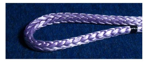
The end of the rope is taped to a metal fid, which is inserted through the strand to form the first lockstitch
