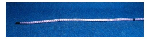
Lay out the rope to the desired eye size
