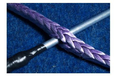
Pull the strand through until the mark for the buried length is completely through
