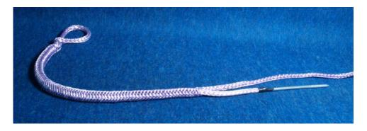
Remove metal fid. One third of the buried length is pulled out in order to taper the end.
