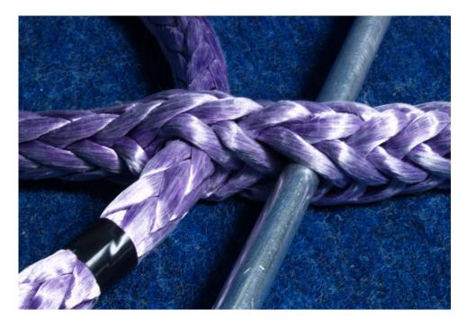
Then skip 2 picks and make the insertion for burying the tail end of the splice.
