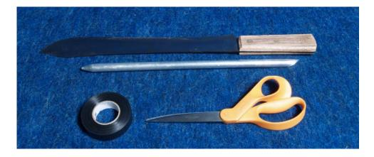
A fid length is determined by multiplying the circumference of the rope to be spliced by 7.1. When splicing ropes such as Plasma and Spectra, 3 fid lengths are buried. Lay the rope out and mark the buried fid length with tape or marking pen.
